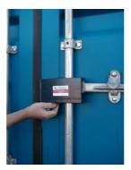
Control of the bolt clamp: Pull the bolt clamp to check that it is in locked position.
