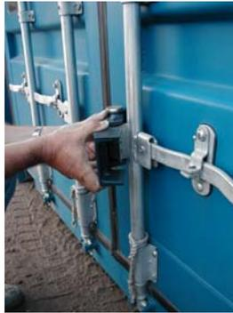
The CC FixCode 1 being fitted above the handle and pressed against the container.
