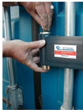
To lock the container, push up the plunger as far as it will go and turn the lock dial four times.
