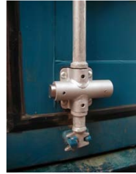
The seal is protected against being broken until the combination has been set correctly.
