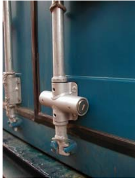
The CC Bearing Bracket 1 can be fitted during manufacture of the containers.
